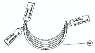
Illustration 6 : Application of sealing compound on the floating labyrinth seal
