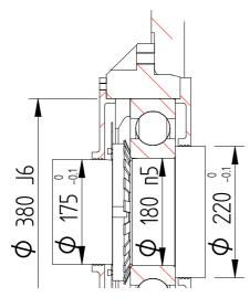
1 - Bearing carrier 2 - Outside bearing cover 3 - Snap ring 4 - Fixed deflector
