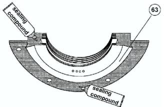
Illustration 10: Application of sealing compound on the rigid labyrinth seal
