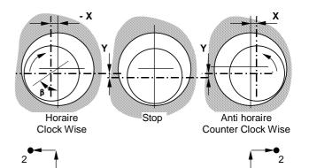
Clear : diametrical clearance Oil film : oil film thickness β : Attitude angle
