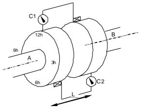
The "C1" and "C2" micrometers are located at an angular difference of 180°.
