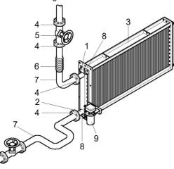
Water pipes must be connected stress free
