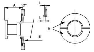
Two half-shells (B parts) mounted on the front flange act as a front bearing for the transportation and installation. The outside of the centring half-shells face a groove machined on the shaft.
