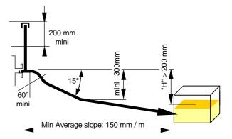
Install a breather as close as possible of the bearing output The breather should be to a minimum of 200 mm above the highest point of the bearing.
