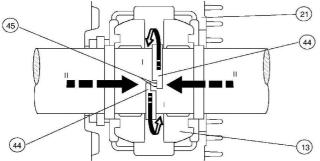
Illustration 5 : Installation of the loose oil ring
