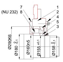
1 - Bearing carrier 2 - Outside bearing cover 4 - Fixed deflector
