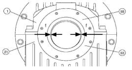
Illustration 11: Alignment of the rigid labyrinth seal Tighten the screws (60) by using the following torque values:
