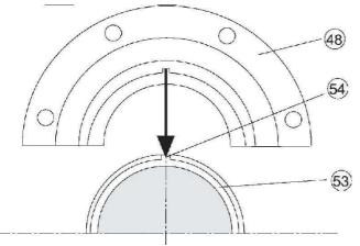
Illustration 9 : Assembly of the seal carrier
