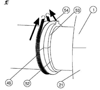
Illustration 7 : Assembly of the floating labyrinth seal Align the split line of the floating labyrinth seal and the split line of the seal carrier.
