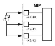
The generator winding temperature V1 can be designed as Pt1000 or Pt100 and is monitored for limit value overshoot and wire break.
