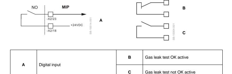
After request for the gas leak test by the MIP 4000, this checkback must be signaled within an adjustable time (e.g. 30 s, parameter is assigned in the MIP 4000) otherwise the start procedure will be interrupted.
