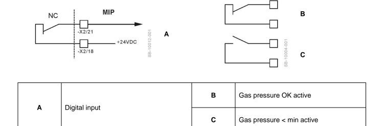
The gas pressure switch "min" must be installed upstream of the gas valves.
