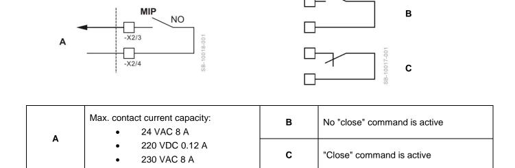
After satisfying the connection requirements the MIP 4000 outputs a close pulse for the generator circuit breaker (GCB). Parameters can be assigned for the pulse length of the close contact (standard: 250 milliseconds).
