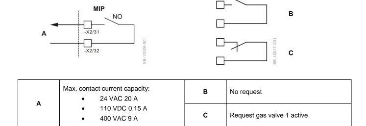
With request the gas valve 1 must open.
