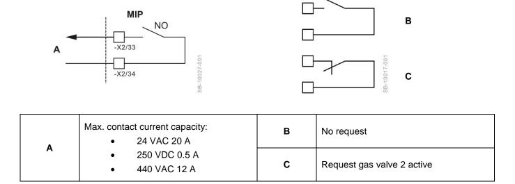
With request the gas valve 2 must open.
