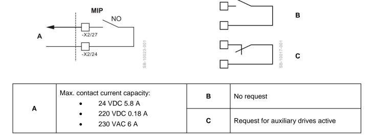
The contact is closed at a start command and will only be opened when the engine is at a standstill and the afterrun time has elapsed.
