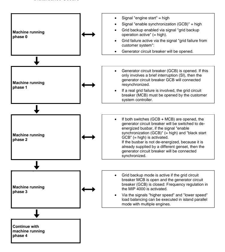
**Machine running** phase 4 Grid backup mode
