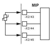
The generator winding temperature W1 can be designed as PT1000 or PT100 and is monitored for limit value overshoot and wire break.
