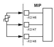
The generator winding temperature - drive side - can be designed as PT1000 or PT100 and is monitored for limit value overshoot and wire break.
