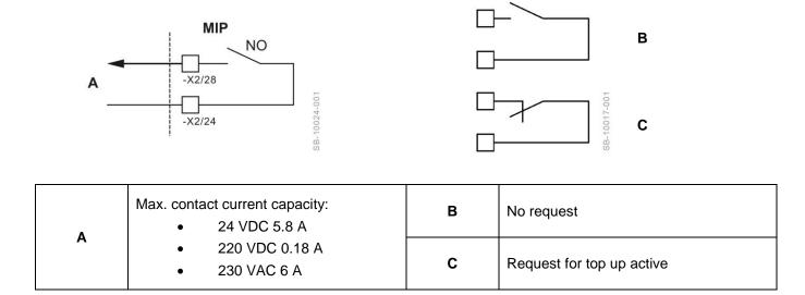
The request for the lubricating oil solenoid valves is activated, if the oil top-up trips due to reduced oil level. The machine must be in operation for at least 5 minutes.
