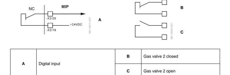
After activation of the output "Request gas valve 2" this checkback must be signaled by the end position switch of the gas valve.
