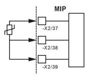
The generator winding temperature U1 can be designed as PT1000 or PT100 and is monitored for limit value overshoot and wire break.
