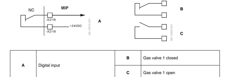
After activation of the output "Request gas valve 1" this checkback must be signaled by the end position switch of the gas valve.
