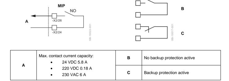
Backup protection is activated when the generator circuit breaker (GCB) cannot be opened by the MIP 4000. In this case the customer system controller must open a higher-level switch.
