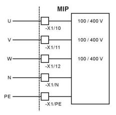
Version 400 VAC or 100 VAC can be used as busbar voltage.
