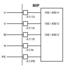
Version 400 VAC or 100 VAC can be used as grid voltage.
