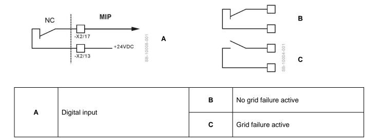
If a grid failure in grid backup operation is detected via this input, the generator circuit breaker (GCB) of the MIP 4000 will be opened.
