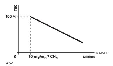
So as to ensure the necessary service lives the silicon content must be checked at regular intervals as part of a comprehensive gas analysis.
