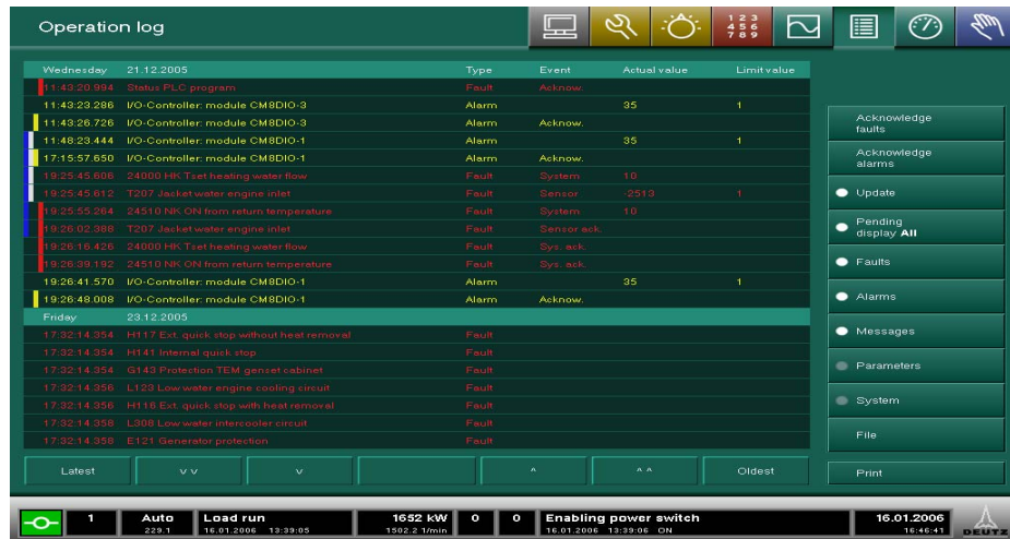
Figure 2: Day changeover operation log
